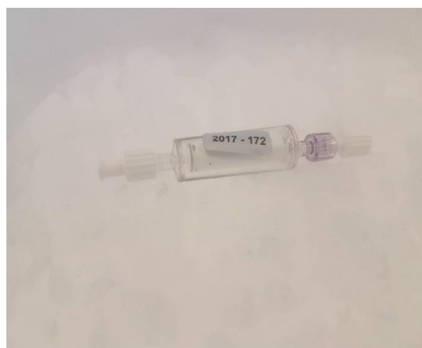
Store the filter on ice (or at -20°C) as soon as possible
