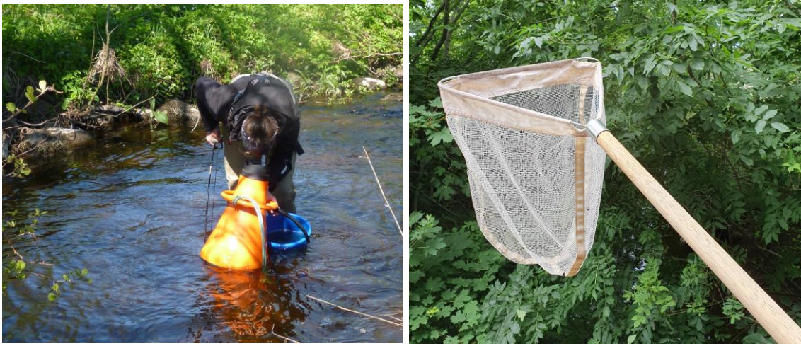
Figure 7. Visual inspection of the river bottom (left) and example of net for sampling sediments (right). Pictures by Sofia Mulla Kølmeel.
